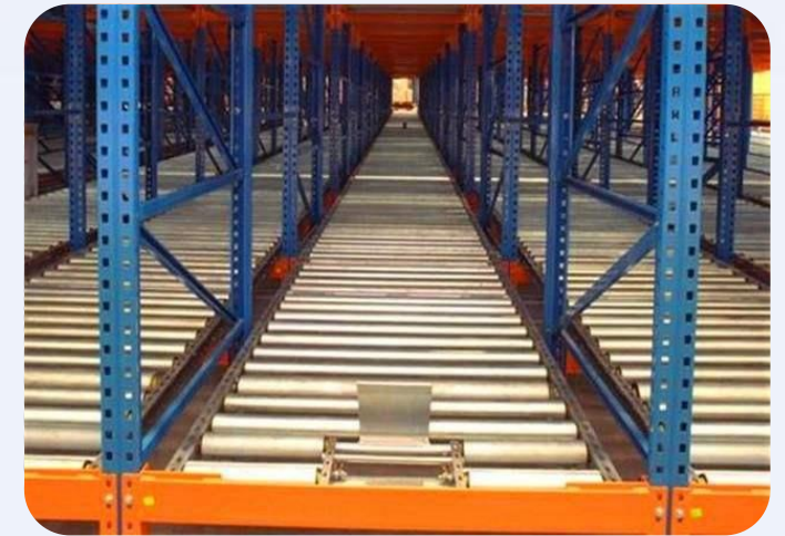
Live Pallet Racking
